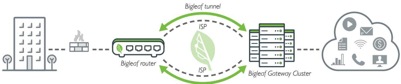
The Bigleaf router installs outside the firewall, prioritizing application traffic in and out of the customer's LAN
